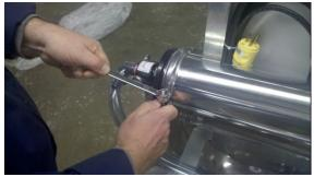
Insert back in the housing the black cap, making sure the pin of the membrane slides in the cap. Notice that it's possible that it will be quite hard to push the cover all the way in.
