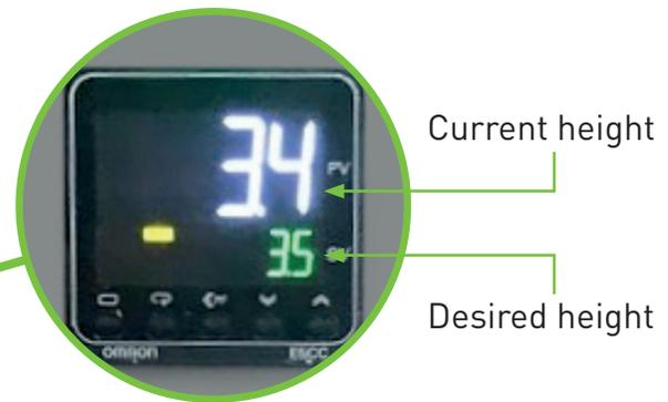
1. Visual indicator for automatic mode (indicator lights up when the switch is set to automatic mode)
