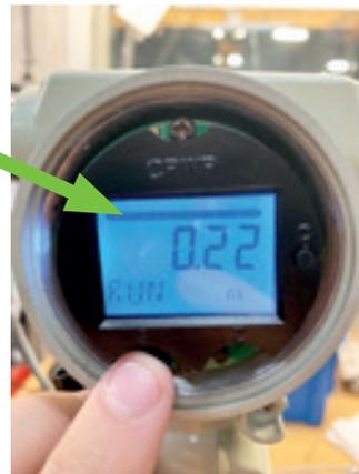
To set your low level, remove water until it reaches -3", then press and hold the S and Z buttons simultaneously for 15 seconds until "Z50K" appears. Once "Z50K" appears, release the buttons and press on the "Z" button (on the right) to record your low level. Afterwards, the black bar like the one in figure 3 will disappear (fig. 4). This means that your low level has been recorded.
