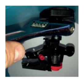
Ensure the rubber gasket is tightened properly with a crescent wrench to prevent leaks.
