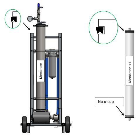
Before removing membranes from the RO system, remove any liquid remaining in the housings using the drain valves. Next, unscrew the collar and remove the upper cover. Lay the system flat and remove the membranes. Do not use pliers to remove the membrane via the filtrate tube! This may damage the tube, causing sugar to run into the filtrate.
