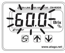
Fig.14-4 Example: When the upper limit value of the recorder output range is set to Brix 60.0%.
