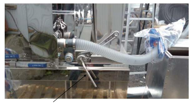
The damper will have to be adjusted between 35 to 45 degrés from the vertical. Magnehelic gauge must read 0.1.
