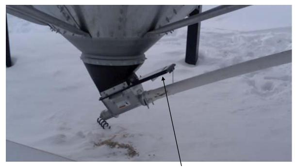
Silo gate valve, only open 1/3 in normal operation
