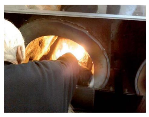
Spray the top of the pellets with fire starter like diesel and lite with a propane torch
