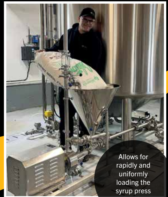
Dynamic Mixer YRL 1-100 with 5.5 HP motor 668429
